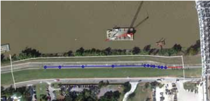
Global stability levee project area plans circa June, 2012. Montage is courtesy of SLFPA-W. Fair use Google Earth Image shows planned project area per engineering drawings courtesy USACE (white outline) with existing sheet pile in red and proposed additional sheet pile in blue just upstream of the cracked levee section on the opposite side of the HPL Bridge.
