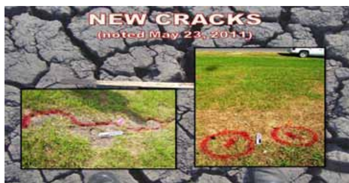
Figure 6: New cracks upslope from the drifting post.
