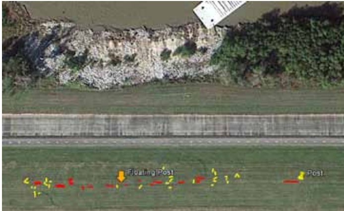
Figure 8: Cracking levee and bank collapse location are the same! Inferred tension cracking in levee crown and protected side extension cracks correspond to two recent flood side bank collapses.
