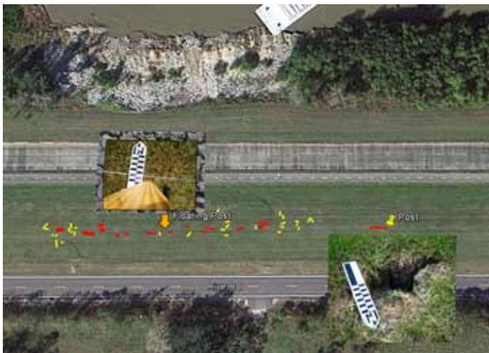
Montage, on fair use Google Earth Base courtesy SLFPA-W, showing May 23, 2011 cracks mapped by Merritt. Note widest, deepest, sometimes 10' long cracks in red, orange arrow showing post "drifting" downslope away from reference string and smaller, perpendicular crack trends in yellow aligned with flood-side slump boundaries.
