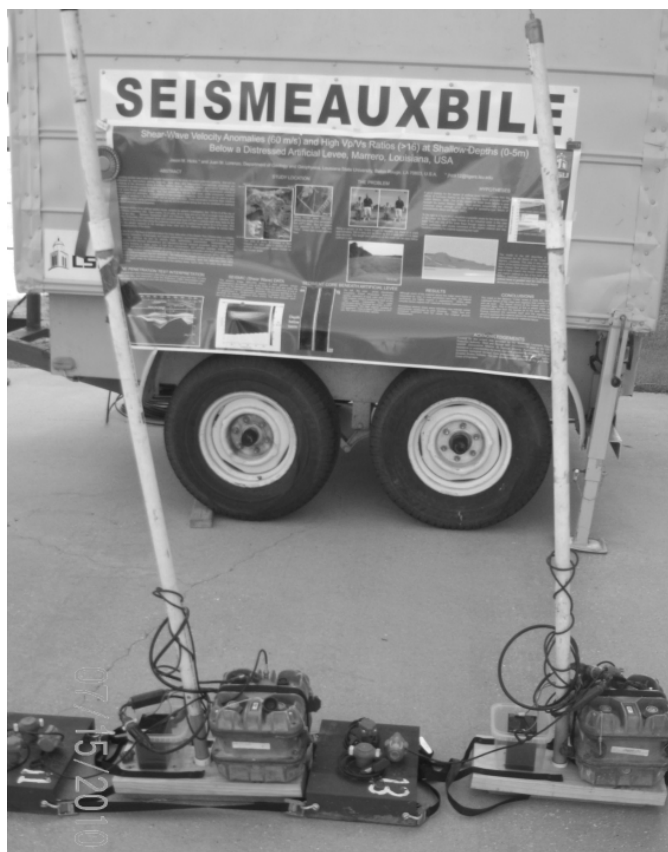
LSU's custom-crafted “Seismeauxmobile” and sound generators displayed at the Fourth NOGS Flood Protection Symposium in Gretna. The research instruments are used to detect weak/problem spots in levees in south Louisiana.
