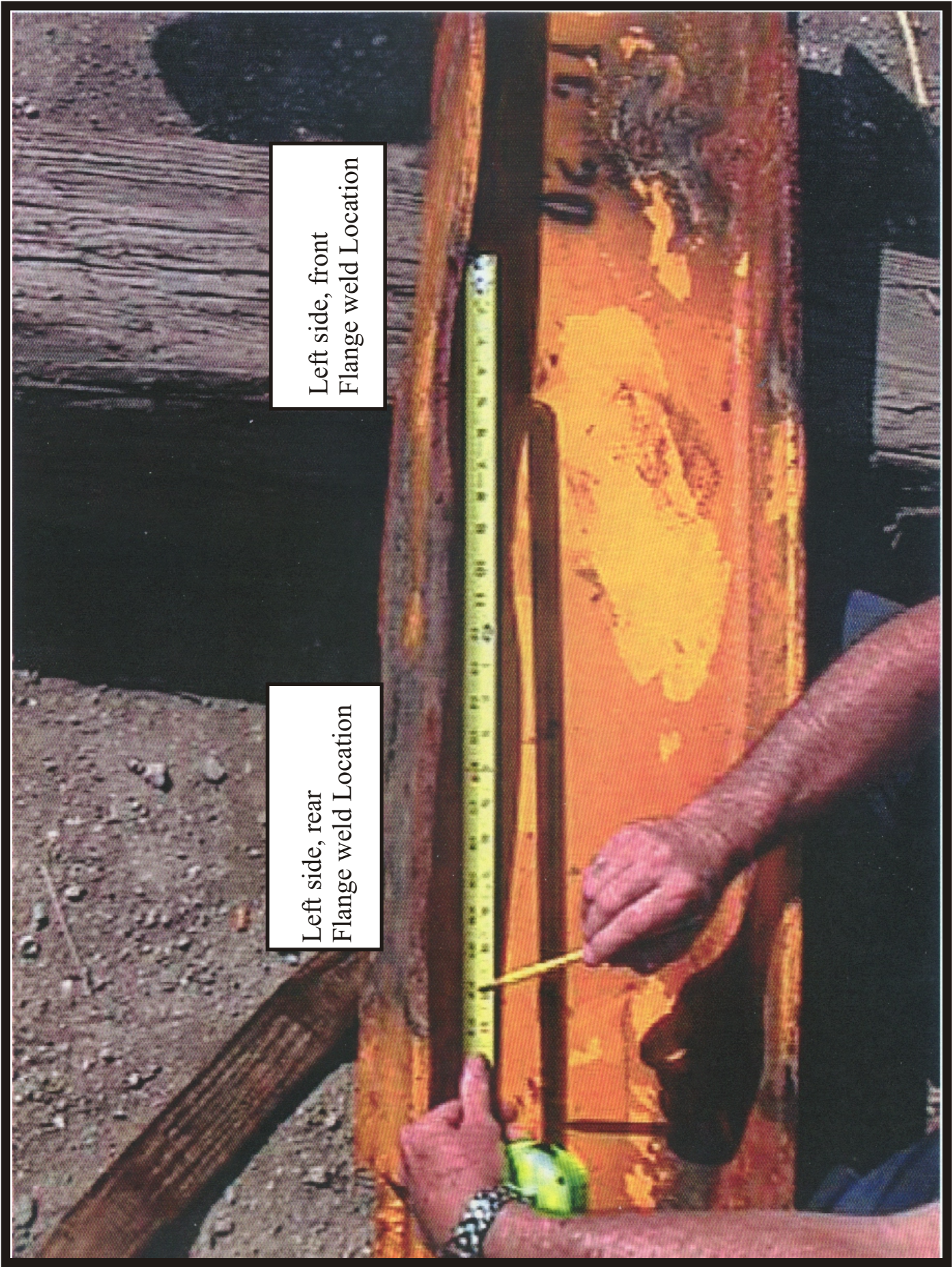
Deformation of I-Beam Flange
