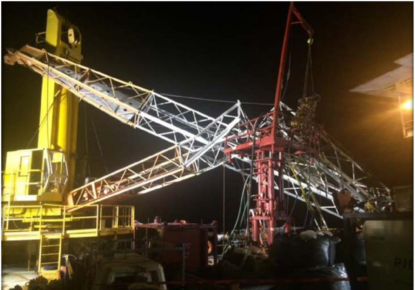
*In two separate incidents, a catastrophic offshore accident was caused in part by the ejection of hydraulic pulling unit (casing jack) traveling slips when a bind on the pipe being pulled was suddenly released.*
